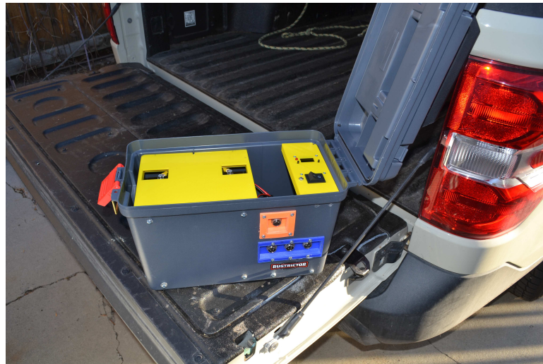
Figure 1: Power supply and monitor/recorder with 30 Ah battery
