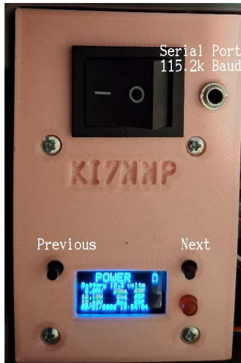
Figure 8: Recorder/monitor Control Panel
